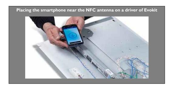
**Step I**: Open the smartphone app downloaded at Google Play. Place the smartphone next to the NFC antenna on the driver (small blue rectangular device located at end of the driver, same end as incoming AC power). The phone app will indicate if it has read the settings on the SimpleSet driver.
